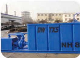
Mud mixing unit
