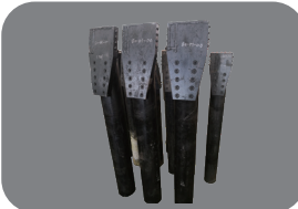
Beacon housing & drill bit
