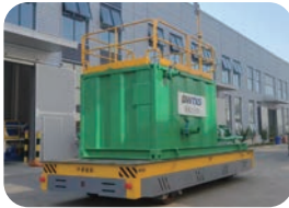
Mud mixing system
