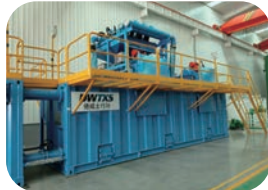
Mud mixing & recycling
