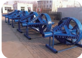
Cutting type Backreamer
