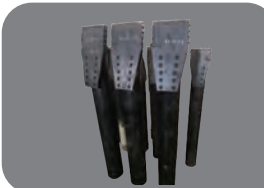
Beacon housing & drill bit
