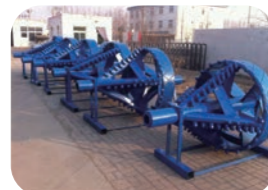
Cutting type Backreamer
