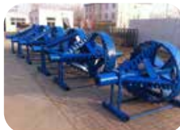
Cutting type Backreamer
