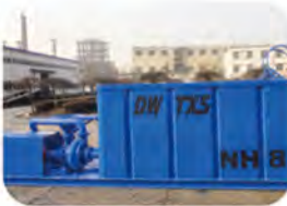
Mud mixing unit
