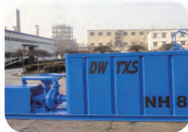
Mud mixing unit
