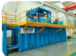
Mud mixing & recycling
