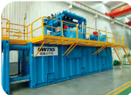
Mud mixing & recycling
