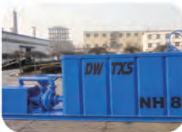
Mud mixing unit
