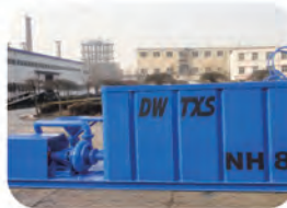
Mud mixing unit
