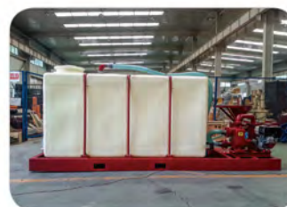
Mud pumping unit form 1 m 3 to 10 m 3
