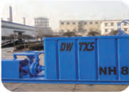
Mud mixing unit
