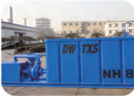
Mud mixing unit
