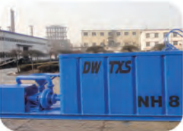
Mud mixing unit
