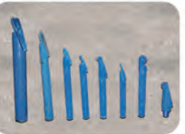
Beacon housing and drill bit
